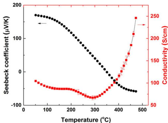
FIG. 5. The absolute Seebeck coefficient and electrical conductivity from 50 to 473 °C for the SLM-processed  $\text{Bi}_2\text{Te}_3$  sample. The conductivity data were averaged over a set of ten measured values, and the uncertainty bar shown is from the standard deviation. The uncertainty on the measured Seebeck coefficient is  $\pm 7\%$ , according to the Linseis technical specifications.
