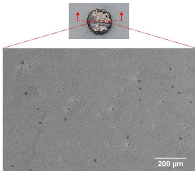
FIG. 2. Scanning electron micrograph of a polished cross section of the SLM processed  $\text{Bi}_2\text{Te}_3$  bulk sample. Each layer is about 150  $\mu\text{m}$  thick; no separation between powder layers is observable.
