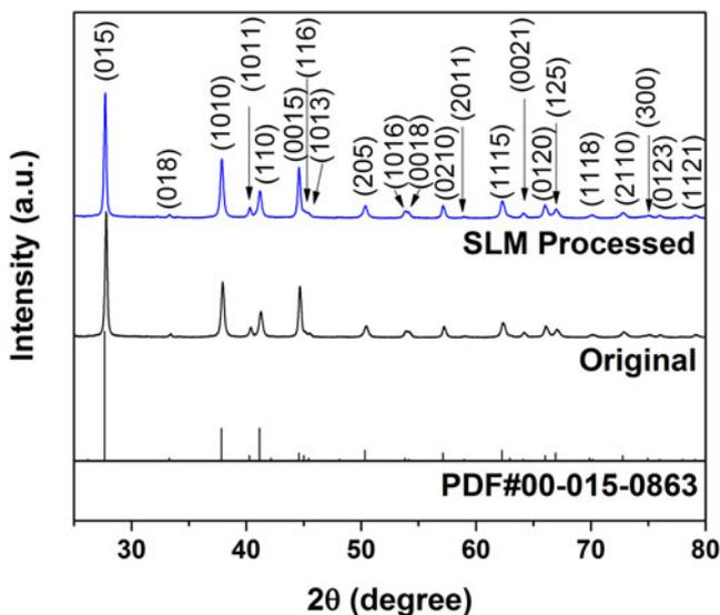
FIG. 3. XRD patterns of  $\text{Bi}_2\text{Te}_3$  samples for original powders and those from SLM processed sample. Both spectra are well-matched with positions and intensities, and they match the database values for  $\text{Bi}_2\text{Te}_3$  (PDF#00-015-0863).
