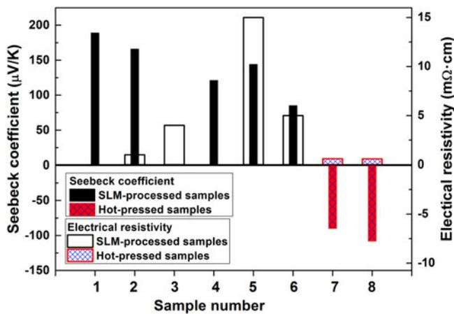
FIG. 4. A summary of the measured Seebeck coefficient and electrical resistivity at room temperature. Samples #1–#6 are the SLM-processed samples; samples #7 and #8 are fabricated through hot-pressed method on pristine powders. The processing parameters for all the samples can be found in Table S1 in the Supplementary Material.
